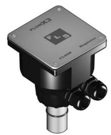
The NEW FLOWX3 F3.60M & F3.63M Insertion Magmeters are suitable to measure flowrate in both metal and thermoplastic pipelines. No moving mechanical parts and the high quality materials allow the measurement of liquids where suspended solids can be present or of abrasive liquids as long as they are conductive and homogeneous.
